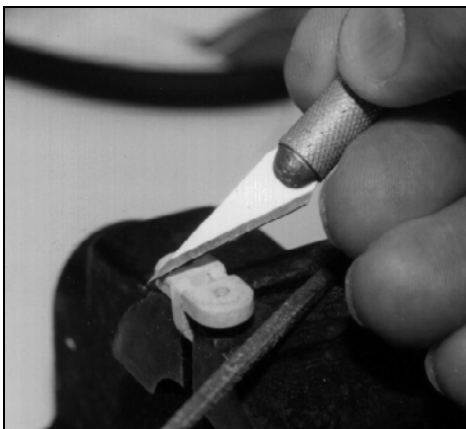
Groove the eyelet to recess the line
